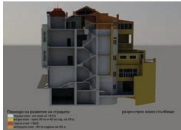
Fig. 10. Vertical section through the right staircase.
